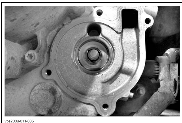
TYPICAL - INNER PART OF ROTARY SEAL REMOVED
