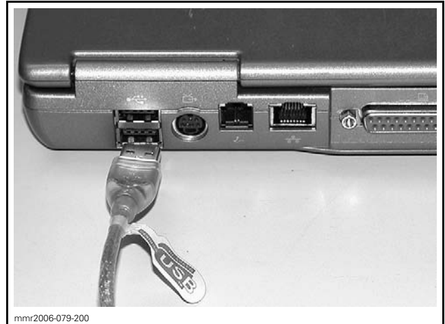
MPI CARD CABLE CONNECTED TO USB PORT
