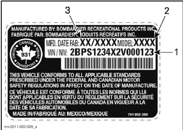
TYPICAL — VEHICLE IDENTIFICATION NUMBER LABEL 1. VIN (Vehicle Identification Number) 2. Model number 3. Manufacturing date
