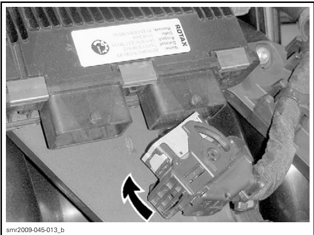
CONNECTOR LOCKING CAM IN RELEASE POSITION
