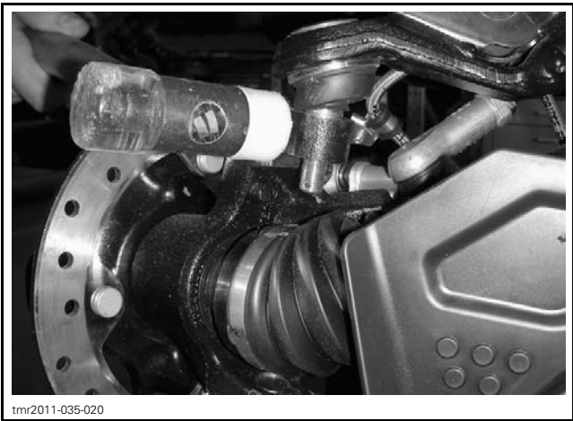
CAREFULLY HIT ON KNUCKLE SIDE
