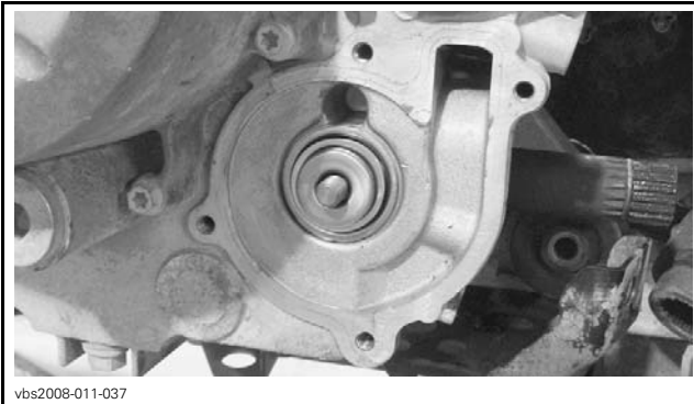
ROTARY SEAL PROPERLY SEATED ON CRANKCASE
