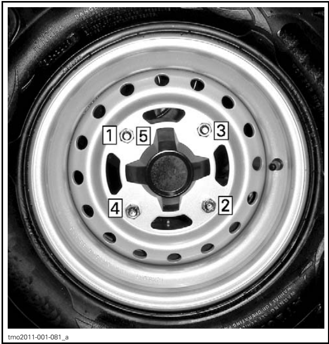
TIGHTENING SEQUENCE
