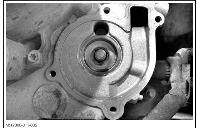
TYPICAL - INNER PART OF ROTARY SEAL REMOVED
